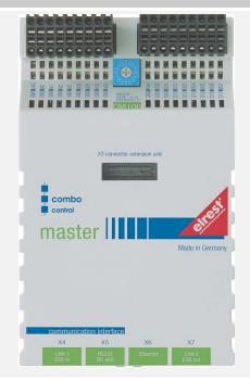
Compact combo master I/O module with integrated soft SPC
